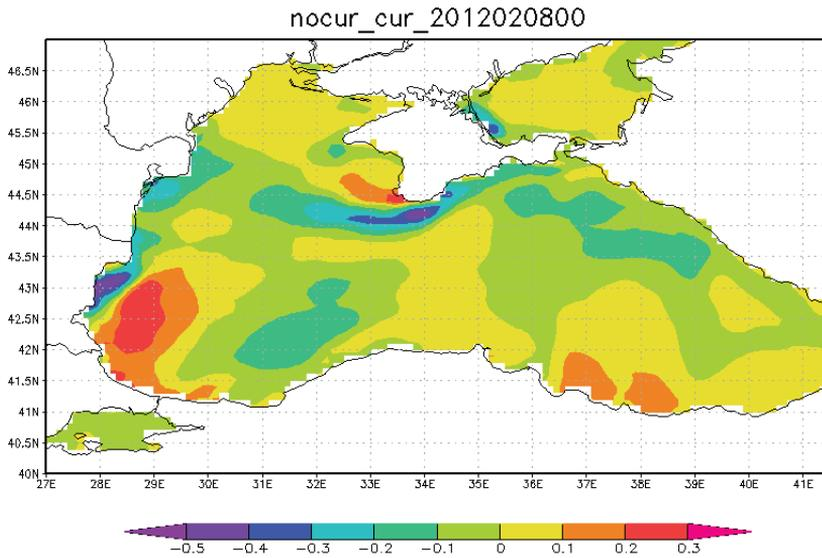
**Fig. 5.** Difference between the modelled significant wave heights for the Black Sea with and without wave-current interaction during the storm of February 2012. SWAN wave model with WAM cycle 4 physics.
