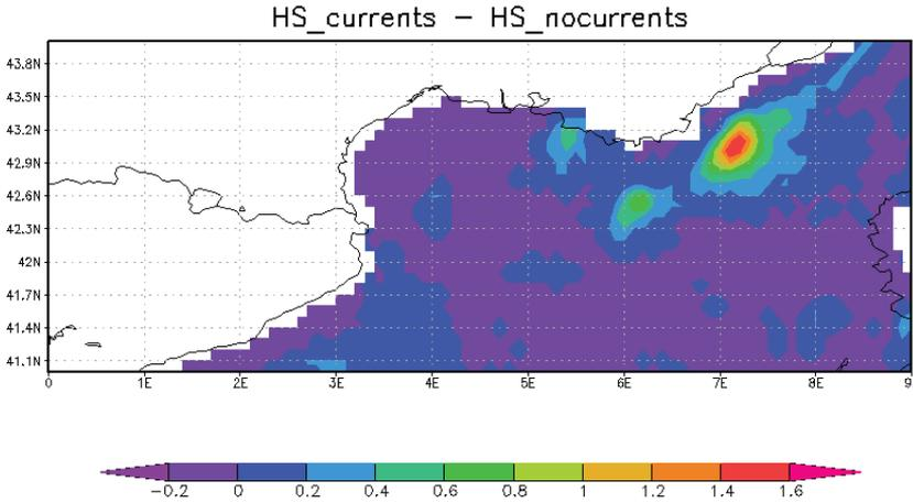
**Fig. 3.** Significant wave height [m] difference between simulations with and without wave-current interactions.
