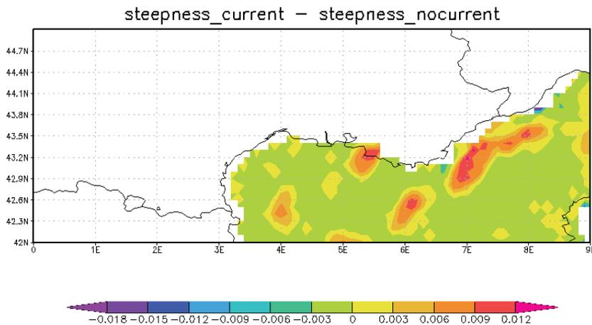
**Fig. 2.** Wave steepness difference between simulations with and without wave-current interactions.
