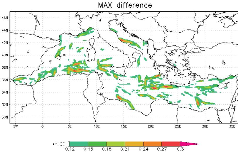
**Fig. 4.** The highest positive differences for the entire October 2014 (MFWAM simulation)- the difference for each 3 hours is taken and then the highest for each grid cell is extracted and plotted.
