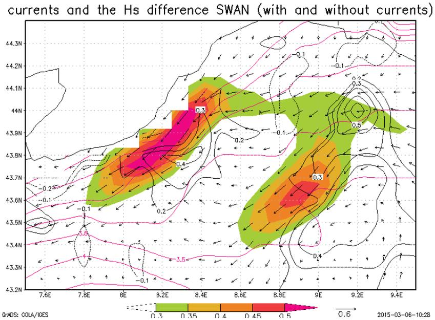
**Fig.1.** Surface currents (vectors), currents speed (black contours), significant wave height without wave-current interaction (purple contours), the difference in significant wave heights with and without wave-current interaction (colour range). Simulation with SWAN for a case in October 2014.
