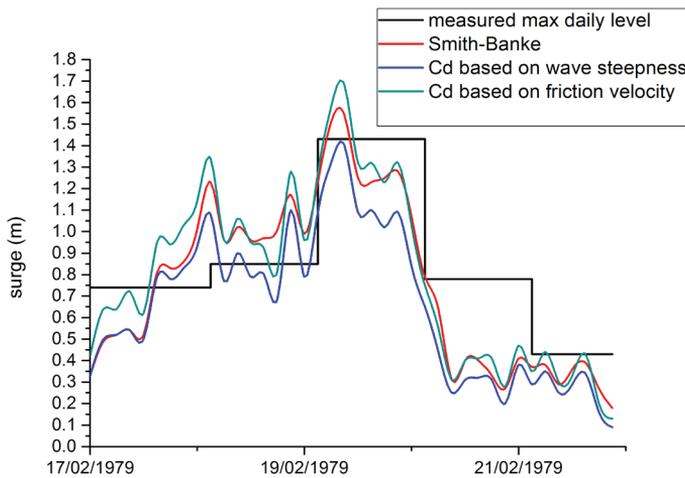
**Fig. 3.** Comparison of the measured daily maximum surge measured at Irakli tide gauge with model simulations using the default Smith-Banke formula and  $C_d$  estimated using the wave steepness and  $C_d$  based on the friction velocity obtained by the SWAN wave model.
