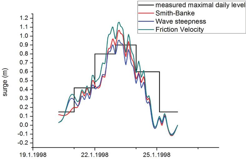
**Fig. 5.** Comparison of the measured daily maximum surge measured at Irakli tide gauge with model simulations for the storm of January 1998 using the default Smith-Banke formula and  $C_d$  estimated using the wave steepness and  $C_d$  based on the friction velocity obtained by the SWAN wave model.
