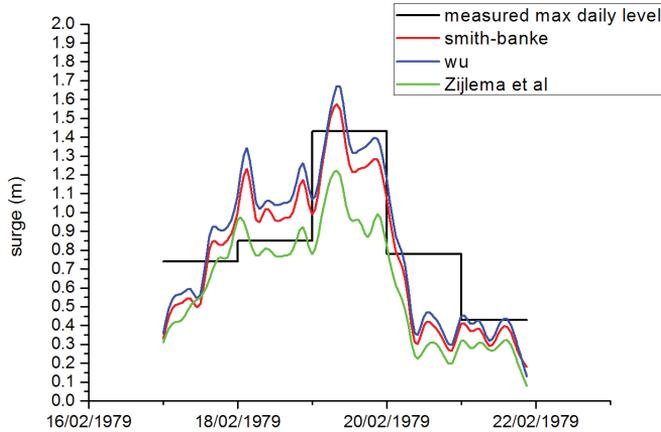
**Fig. 2.** Comparison of the measured daily maximum surge measured at Irakli tide gauge with model simulations using Smith-Banke and Wu bulk parameterizations of  $C_d$  and the second order bulk formula of Zijlema et al (2012).
