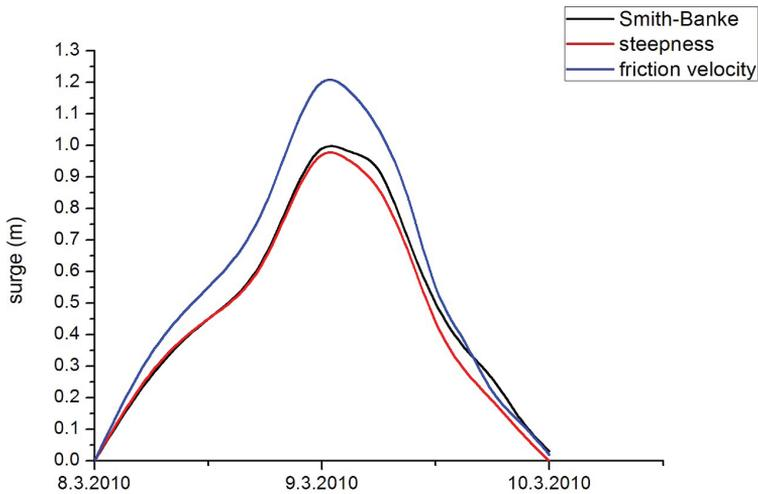
**Fig. 6.** Model simulations using the default Smith-Banke formula and  $C_d$  estimated using the wave steepness and  $C_d$  based on the friction velocity obtained by the SWAN wave model- the storm of March 2010.
