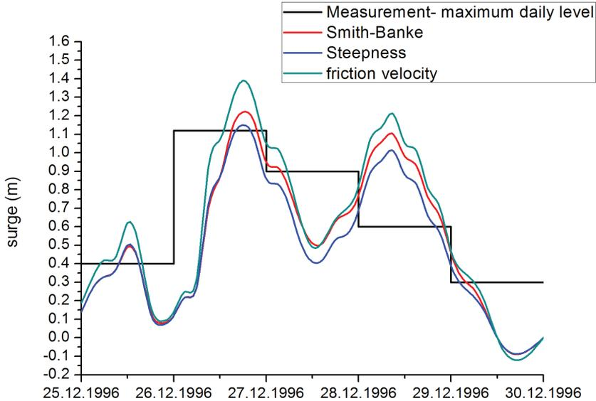
**Fig. 4.** Comparison of the measured daily maximum surge during the storm of December 1996 measured at Ahtopol tide gauge with model simulations using the default Smith-Banke formula and  $C_d$  estimated using the wave steepness and  $C_d$  based on the friction velocity obtained by the SWAN wave model.
