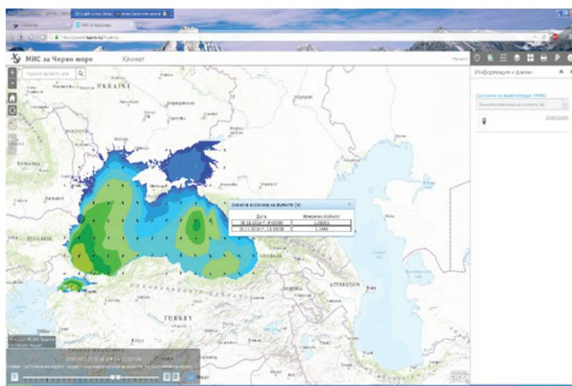
**Fig. 4.** User interface of web based GIS application in MISBS showing modelled SWH and wave direction for the Black Sea (Demonstration of image zooming capability and generation data at selected point)
