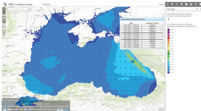
**Fig. 3.** User interface of web GIS based application in MIBS showing SWAN simulation results for the Black Sea (at the bottom left is the Time Slider window and on the right – table with time evolution of significant wave height at selected point)
