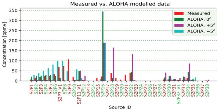
**Fig. 3.** Comparison between ALOHA’s estimated (0°, +5° and –5°) and wind tunnel measured concentrations [ppmV] for source S2
