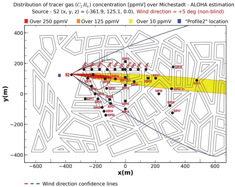
Fig. 2. Wind direction sensitivity of ALOHA; top is for  $0^\circ$ ; middle for  $-5^\circ$ ; and bottom for  $+5^\circ$
