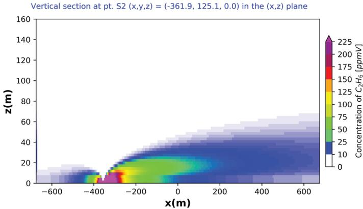
Fig. 8. AERMOD estimated concentration distribution of ethane – a vertical section.
