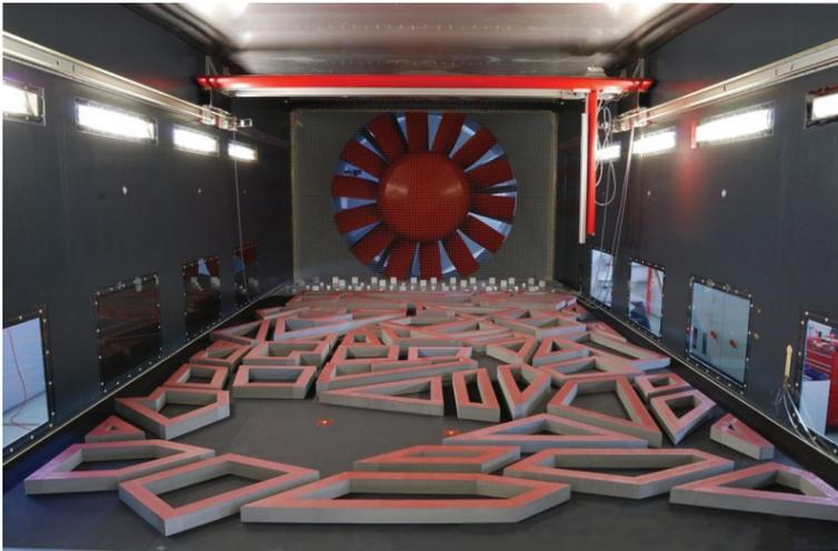
**Fig. 1.** “Michelstadt” urban layout developed in the wind tunnel “WOTAN” and used for model evaluation.
