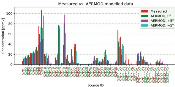
Fig. 9. Comparison between AERMOD's estimated (0°, +5° and -5°) and wind tunnel measured concentrations [ppmV] for source S2
