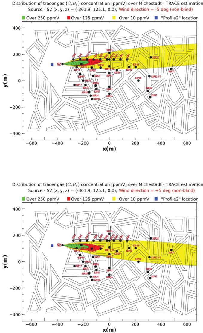
**Fig. 5.** Wind direction sensitivity of TRACE; top is for  $0^\circ$ ; middle for  $-5^\circ$ ; and bottom for  $+5^\circ$
