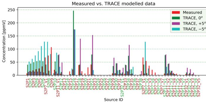
**Fig. 6.** Comparison between TRACE’s estimated ( $0^\circ$ ,  $+5^\circ$  and  $-5^\circ$ ) and wind tunnel measured concentrations [ppmV] for source S2
