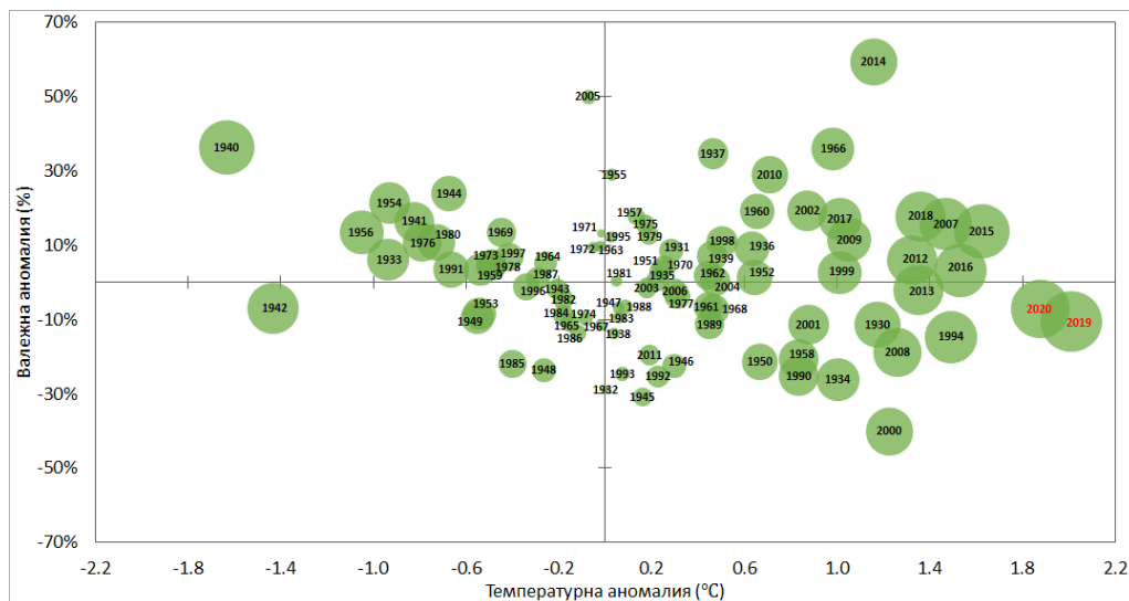
Fig. 4-1 Combined diagram of anomalies of the country averaged annual temperature and precipitation (reference period: 1961-1990). The size of the bubbles is proportional to the absolute magnitude of the temperature anomaly.
