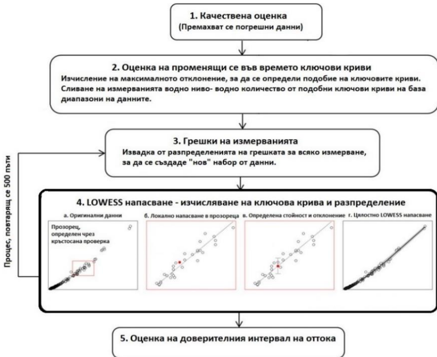
Fig. 4. Schematic representation of the generalized framework for uncertainty estimation. [Coxon et al., 2015]
